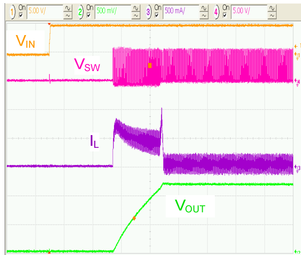
Figure 4. Startup with 100mA Resistive Load
