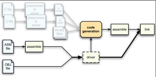
FIGURE 4-4: COMPILATION SEQUENCE WITH ASSEMBLY FILES
