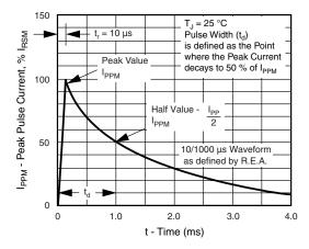
Fig. 3 - Pulse Waveform
