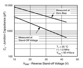
Fig. 4 - Typical Junction Capacitance
