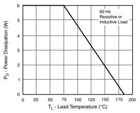
Fig. 6 - Power Derating Curve
