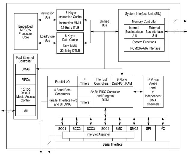
Figure 1. MPC866P Block Diagram
