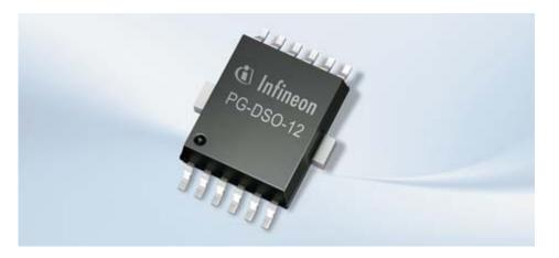
The BTS 500x0-1EGA family consists of single-channel high-side power switches in a green and robust PG-DSO-12-16 package with ON-state resistance (R  $_{DS(on)}$ ) ranging from 5 to 8 m $\Omega$ . The devices offer package, pin and functional (protection and diagnostic) compatibility amongst each other with scaling of R  $_{DS(on)}$  and related parameters.
