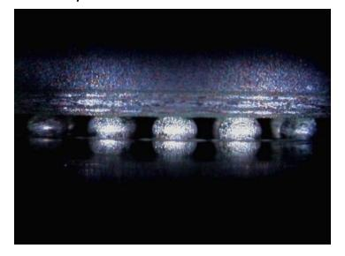
In the photos samples above, trained technicians and computer camera recognition equipment are used for inspection of the X-ray results, looking for voids, shorts, missing connections, contaminants, alignment or other gross failure mechanisms. For example, in Figure 18-20, the BGA ball connections appear to be squashed downward, with mild distortion, insuring that proper oven profile temperatures were achieved.
