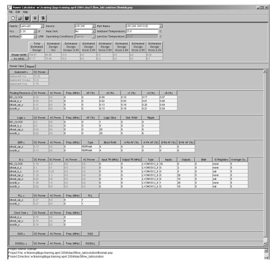
The top pane of the window shows information about the device family, device and the part number as it appears in the Project Navigator. The  $V_{CC}$  used for the Power Calculation is also listed. Users have an option to provide the ambient temperature, and the junction temperature is calculated based on that.
